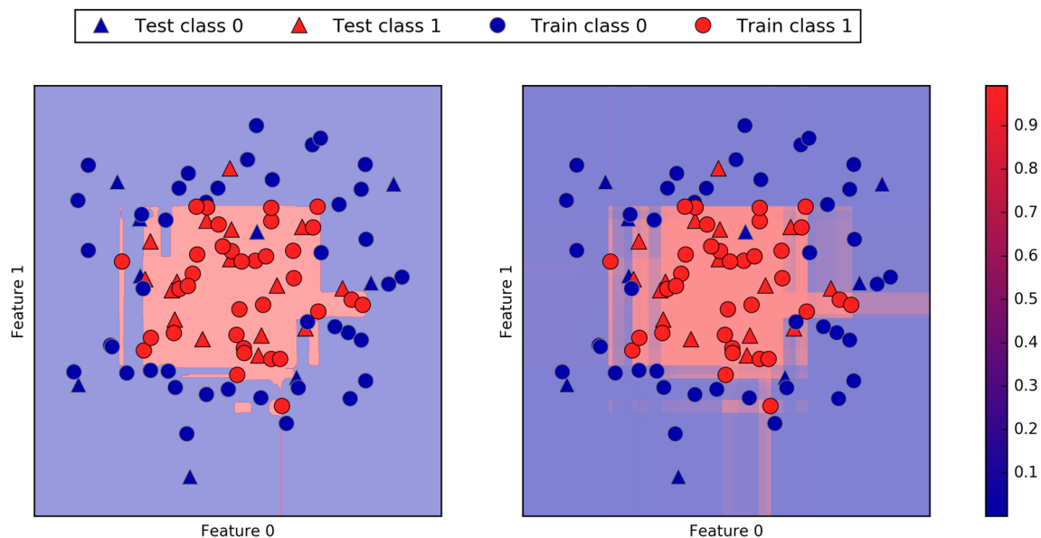
Figure 2-56. Decision boundary (left) and predicted probabilities for the gradient boosting model shown in Figure 2-55
